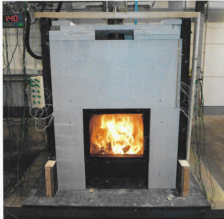
Map. 5 Test installation of the first test - Installation is heated dry (still with open convection air channels)
